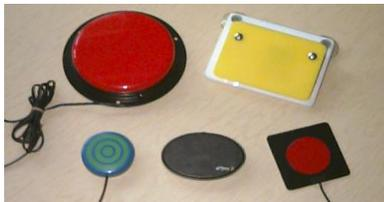
The push (or touch) switch is the most common type, as the child activates the switch by pushing against the surface of the switch. Push switches are available in a wide range of sizes and shapes, in the type of feedback and in the amount of force a child must use.
